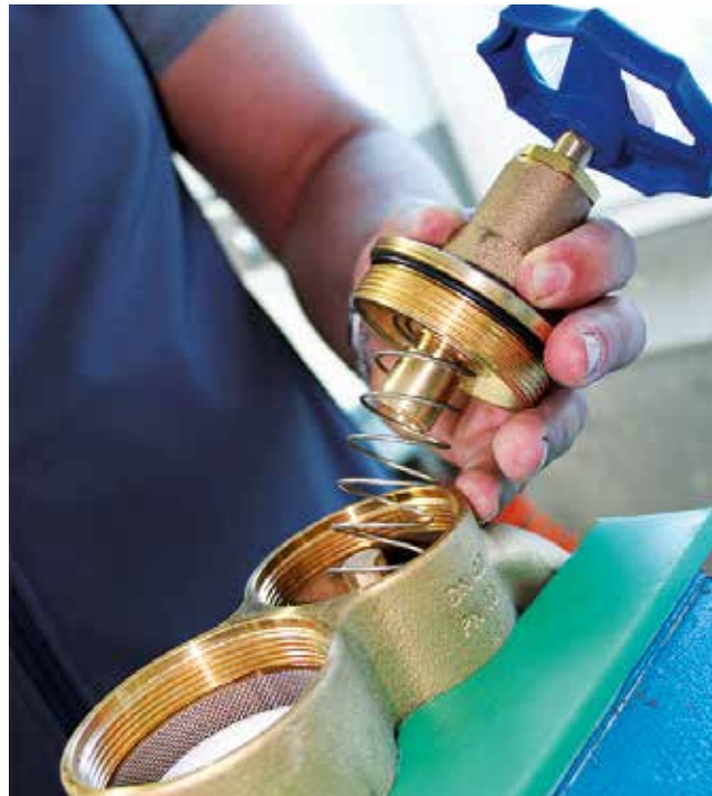
Cleaning and replacement of the individual parts
